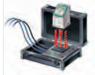
Transmitter Test by flow simulation
