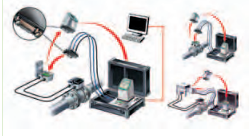
Verificator connection on the SITRANS F M MAGFLO flowmeter
